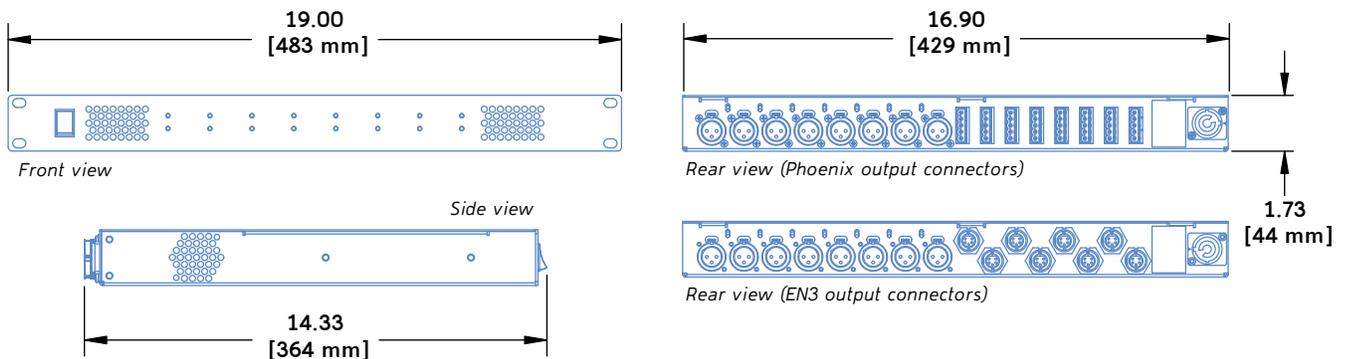
The MPS-488HP IntelligentDC power supply delivers power and balanced audio to up to eight Meyer Sound loudspeakers that require an external DC power supply. The single-space 19-inch rack MPS-488HP can be used with a number of products that feature IntelligentDC technology, such as: the UP-4XP ultracompact loudspeaker, MM-4XP miniature loudspeaker, MM-10XP miniature subwoofer, and HMS-10 surround loudspeaker.
